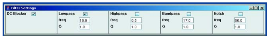
Figure 8. The 'Filter Settings' window allows configuration of the infinite impulse response biquad filter, implemented in software.
