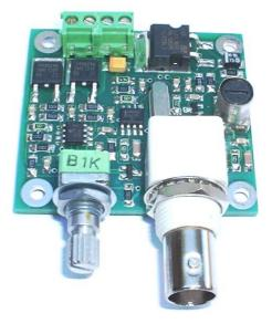
**DESCRIPTION:** The R982A height control is an interface between metal ring surrounding the Oxy cutting torch and drive system for up and down movement of the torch lifter.
