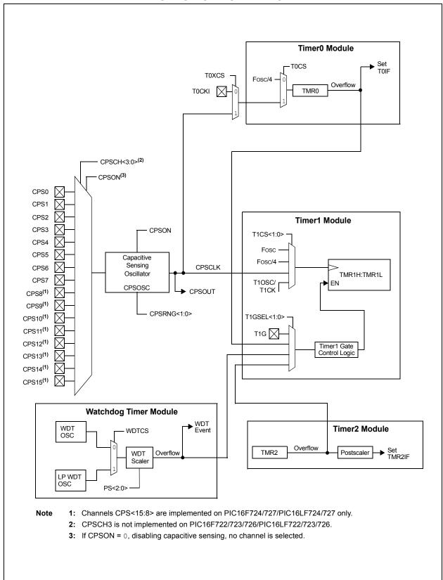
APPENDIX A: CAPACITIVE SENSING BLOCK DIAGRAM
