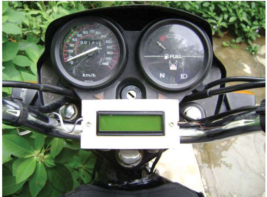
Fig. 6: Speedometer-cum-odometer unit on a bike's handle bar
