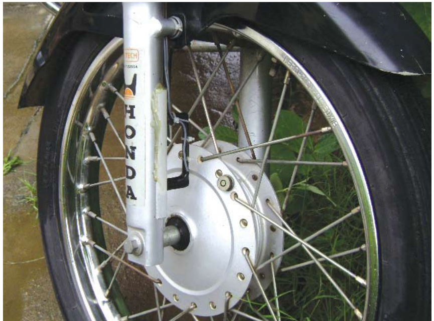
Fig. 5: Reed switch and magnet fixed on the front wheel of motor bike
