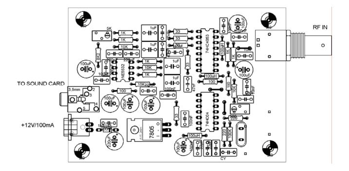
Parts placement for internal oscillator, PCB size 97 x 70 mm
