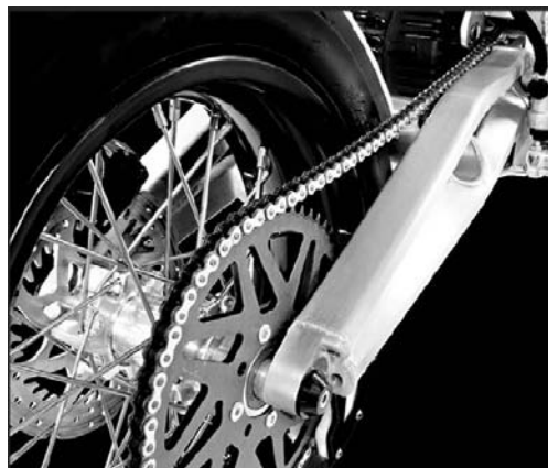
FIGURE 13-9 ZERO electric motorcycle chain drive. ( www.zeromotorcycles.com/gallery.php .)
