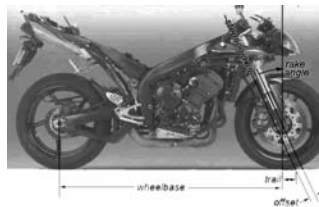
FIGURE 5-2 Picture of bike front headstock angle in relation to ground. (Courtesy of Chris Loughurst, www.carbibles.com/suspension_bible_bikes.html .)
