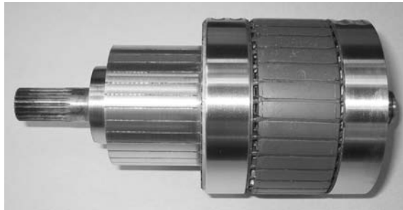
FIGURE 8-9 Photograph of a simple commutator.
