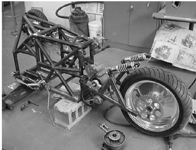
FIGURE 13-8 Transmission placed on prototype 1 swingarm.
