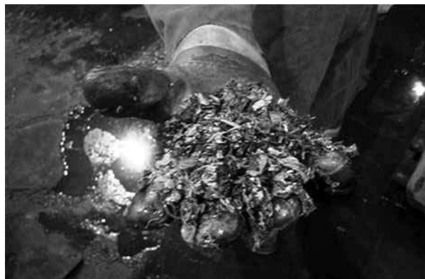
FIGURE 7-31 Tesla electric car battery pack being recycled and reclaimed. ( www.treehugger.com/tesla-battery-recycled-002.jpg .)
