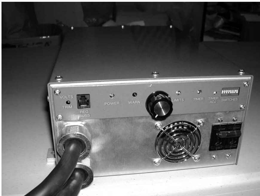
FIGURE 10-8 Manzanita Micro PFC-20, an extremely versatile battery charger. (From Build Your Own Electric Vehicle , Figure 9-4, p. 219.)
