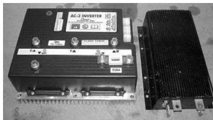
FIGURE 9-32 ZAPI AC3 ac controller size compared with the Curtis 1231.
