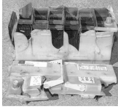
FIGURE 7-24 Battery explosion resulting from gassing.
