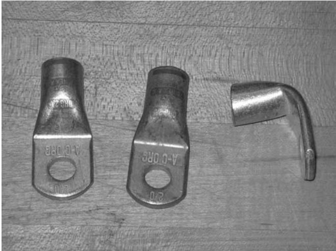
FIGURE 12-10 2/0 terminal ends used to connect to the controller or motor.
