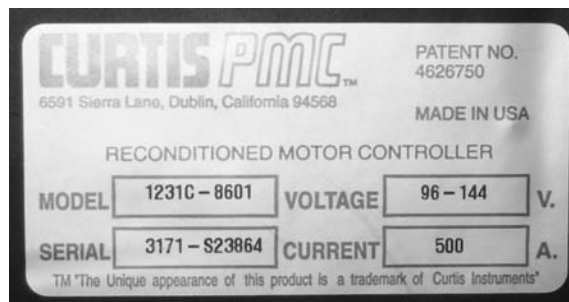
FIGURE 9-7 Curtis controller tag specifications for the Model 1231C.
