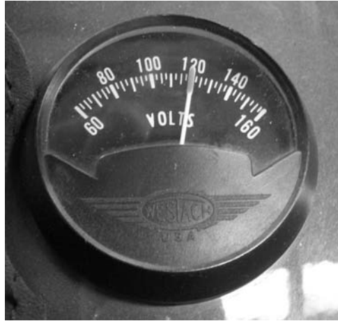
FIGURE 11-8 Voltmeter used on the Electra Cruiser. ( www.westach.com/gauge_images/2C6-30.gif .)
