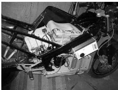
FIGURE 4-2 Electrocat batteries and electric motor. ( evahakansson.se )
