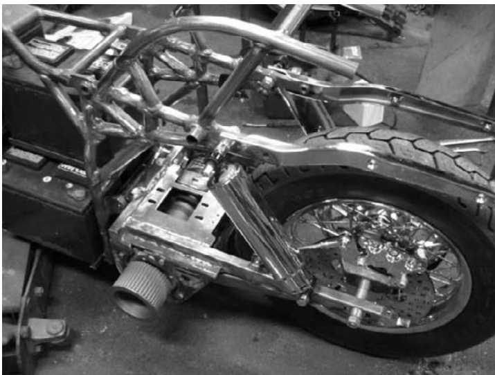
FIGURE 13-12 Fitting the motor to the swingarm.
