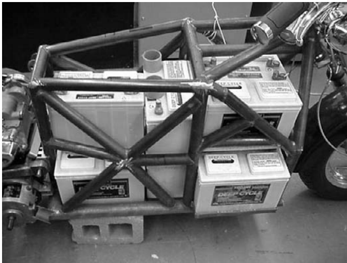
FIGURE 13-16 Fitting 10 Group 27 batteries in prototype 1.
