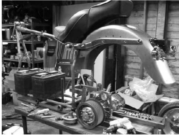
FIGURE 13-7 Fitting the transmission to the swingarm.
