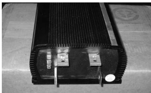
FIGURE 9-16 View of Curtis Model 1231 series connections. ( www.curtisinst.com/index.cfm?fuseaction=cProducts.DownloadPDF&file=50003%5F1221C%2D1231C%5FRevD%2Epdf .)
