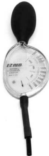
FIGURE 7-22 Inexpensive plastic hydrometer for measuring specific gravity.
