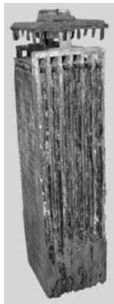
FIGURE 7-14 Sulfation of battery plates. ( www.surfacematerials.com/Cell_sediment.jpg .)
