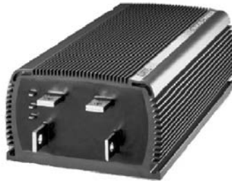
FIGURE 9-6 Curtis Model 1231C 15-kHz PWM controller.
