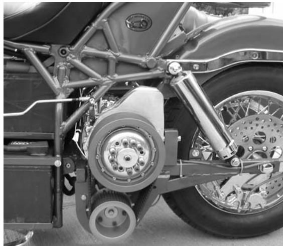
FIGURE 13-14 Clutch basket and belt configuration.
