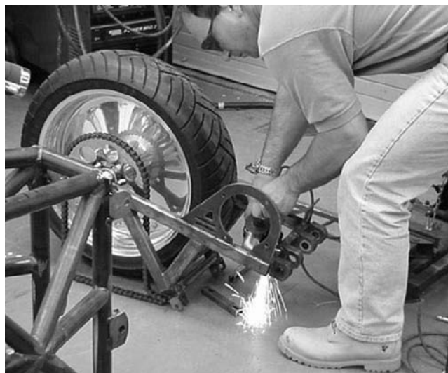
FIGURE 13-10 Modifying the motor mount on the rear swingarm.
