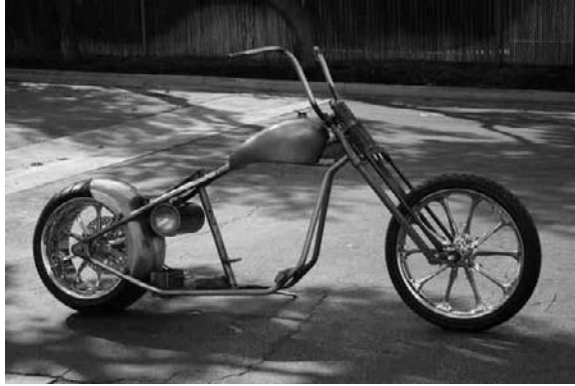
FIGURE 5-3 Rolling frame with reference to height and ground.
