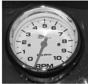
FIGURE 11-11 Electra Cruiser prototype 3 tachometer for use with 10,000-rpm ac motor.
