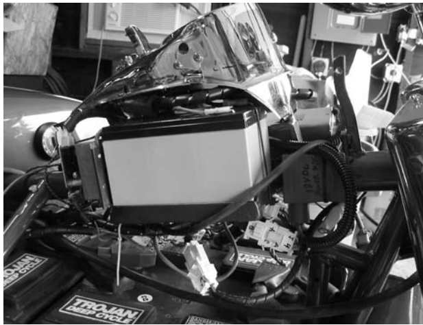
FIGURE 13-20 Inside view of mock tank showing gel battery and PB-6 pot box.
