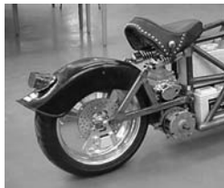
FIGURE 5-18 Hybrid swingarm design: First-generation Electra Cruiser.
