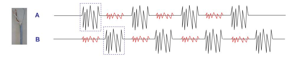
A/B communication is a 16.7 kHz signal sent alternatively on the (A) and on the (B) line. Both signals must match at the other end of the line for the command to be understood.
