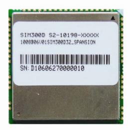
The SIM300D is a complete Tri-band GSM/GPRS solution in a SMT module which can be embedded in the customer application.
