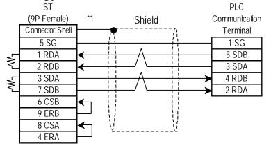
\*1 Be sure to connect the shield to the Connector Shell. For information about FG connections, refer to page 1-2 "RS422 I/F (ST400)" section's Note, in the "Connecting a Device/PLC to the ST unit."
