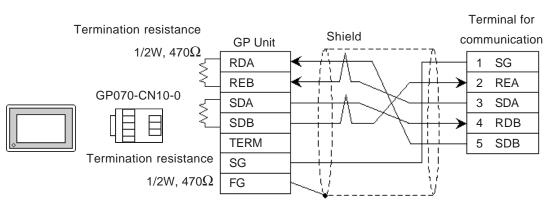
• When using Digital's RS-422 Cable, GP230-IS11-0
