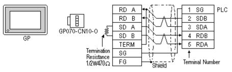
• When using Digital's RS-422 Cable, GP230-IS11-0
