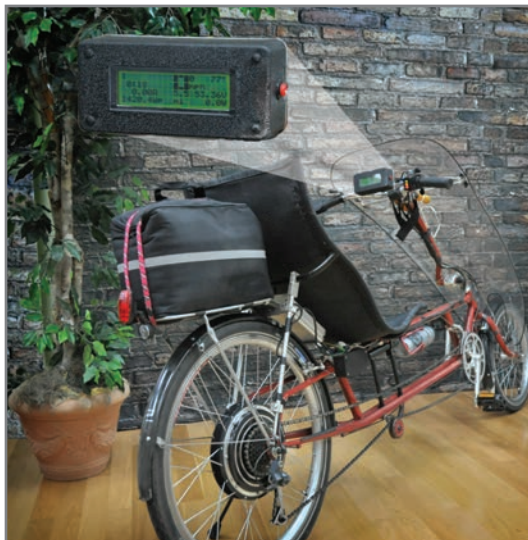
Photo 1 —The EBikeMeter is mounted on an electric-assisted recumbent bicycle's handlebar.
