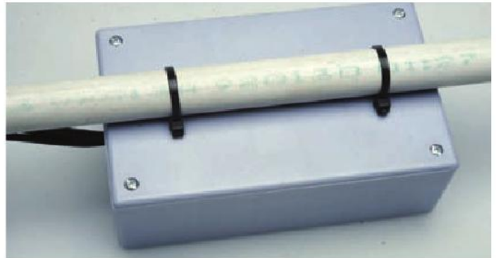
The lid is secured to the PVC pipe by means of a couple of cable ties. When these are pulled tight, they really grip well! Then the lid (which is effectively now the base) is screwed onto the box – and presto!
