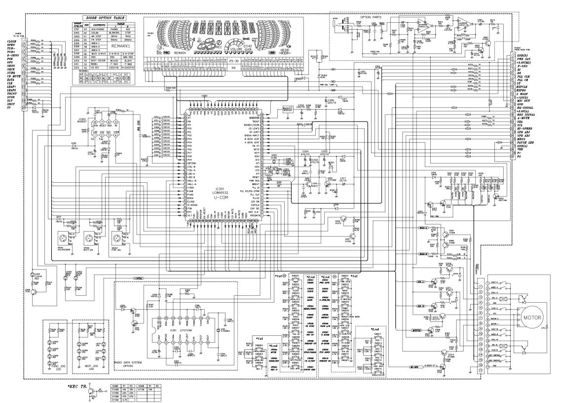
NOTES: Resistance values are indicated in ohms unless otherwise specified (K=1,000, M=1,000,000). Capacitance values are shown in microfarads unless otherwise (P=MICRO-MICRO FARADS). Schematic diagram for this model are subject to change for improvement without prior notice.
