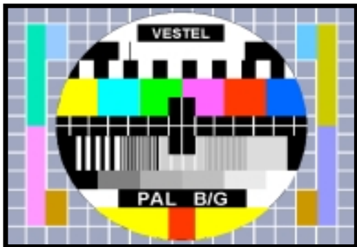
50 Hz. 14:9 Geometry Adjustment for 16:9 Tube
