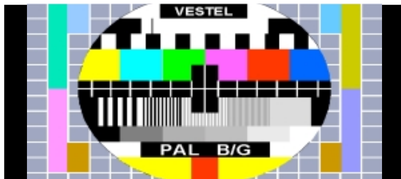
50 Hz. 14:9 Geometry Adjustment for 16:9 Tube
