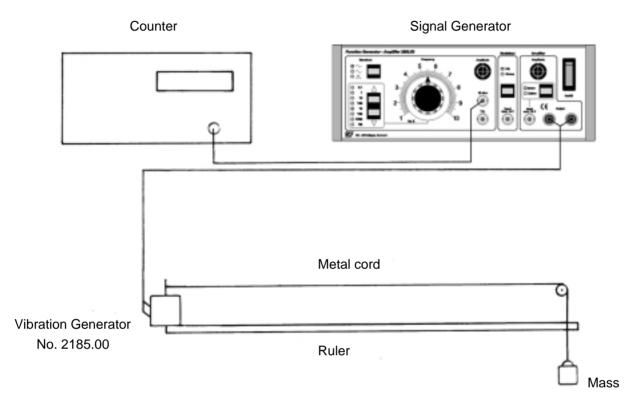
By repeating the experiment several times with different frequencies, it can be demonstrated that the velocity of propagation is independent og the frequency.
