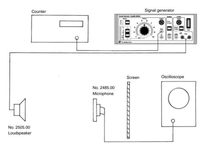
Vaiations in the sound intensity (variations in the height of the curves on the oscilloscope) may be observed by placing the microphone various places between the loudspeaker and the screen. Thus demonstrating that the sound is reflected by the screen ind interferes with the forthcoming wave, resulting in standing waves. A graphic illustration of the results may also be drawn. The experiment may be extended by using screen of different materials e.g. mineralfibre, etc.
