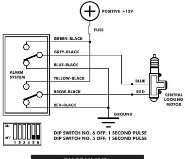
DIAGRAM "2/D" CONTROL FOR ELECTRO-PNEUMATIC MOTOR
