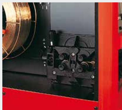
/ Perfect wirefeed thanks to 4-roller drive.
