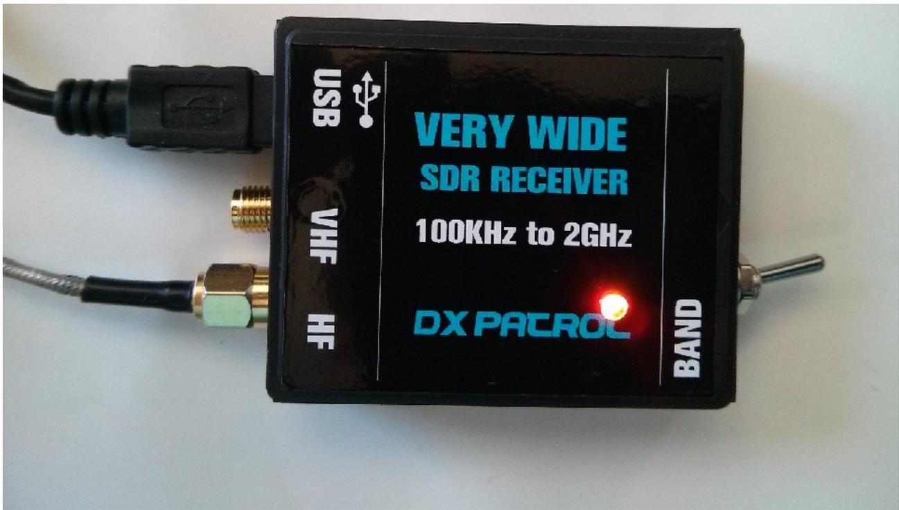
Toggle switch will select the SMA antenna input.
