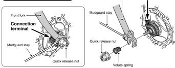
Note:Do not use the toothed axle washer with a quick release type · Connect the two wires to ensure that the current flows smoothly.
