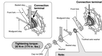
Note: When tightening the cap nuts, tighten the nuts alternately on both sides and do not concentrate all of the effort for tightening and lossening the cap nut on one side of the wheel only, otherwise the hub axle may turn, which could excessively tighten or lossen the lock nuts.
