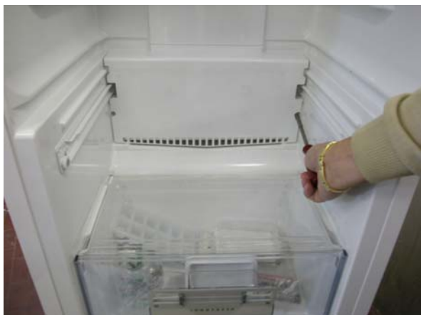
d) remove the 2 fixing screws of the evaporator shield;
