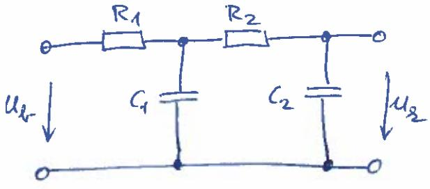
$$Y(s) = \frac{U_x(s)}{U_{x_0}(s)} = \frac{\frac{1}{sC_2} \times \left( R_2 + \frac{1}{sC_1} \right)}{R_1 + \frac{1}{sC_1} \times \left( R_2 + \frac{1}{sC_2} \right)}$$
