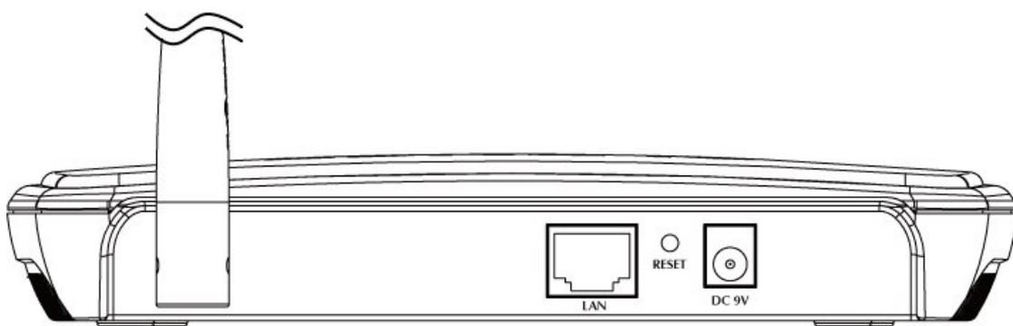
**Power (DC 9V):** The receptacle where you plug in the power adapter.
