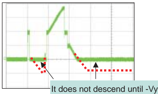
<When the Pass Top FET is damaged>
