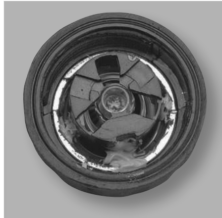
Silicone sealant is also used to secure the collimator lens inside the front assembly of the torch.
