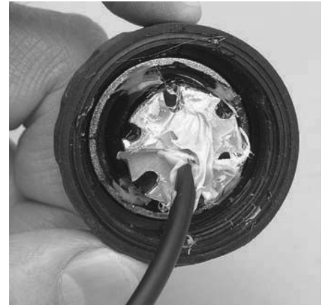
The 1W white LED is then clipped into the collimator lens and secured using additional silicone sealant.
