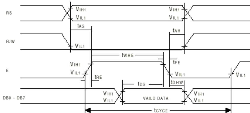
Figure 2. Bus Write Operation Sequence
