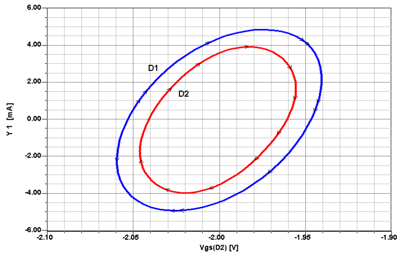
Figure 44--Load lines for the "tuning diodes" D1 and D2, which in reality are GaAsFETs with source and drain tied together. The round shape indicates that the "varactors" are both operating in their linear regions, but the devices themselves are highly nonlinear.
