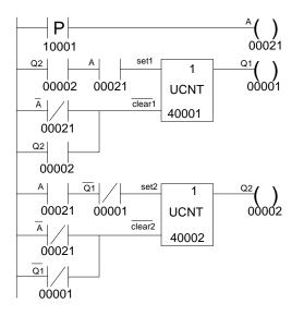
**Step #6:** Program in the above circuit and verify that  $Q_1Q_2$  pass through the states  $00 \rightarrow 01 \rightarrow 11 \rightarrow 10 \rightarrow 00 \rightarrow \dots$  each time SW1 pulses high.
