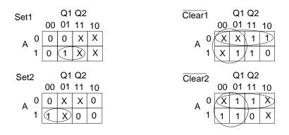
For example, if you are in state 00 (A) and the input is 0, you want to remain in state 00. This means that Set should be zero and Clear can be anything. This is denoted as Set=0 and Clear=X in the upper left corner of each map.
