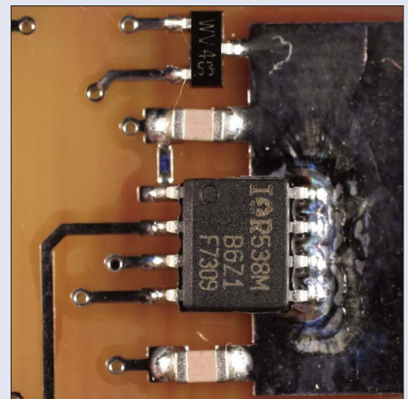
PHOTO 4. Here's a complete half-bridge, including the back-EMF steering diodes and the EMI capacitors. The IRF7309 was designed to switch things about in laptop computers and other electronic devices that require higher switching currents from smaller footprint components.
