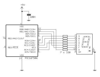
The common cathode pins are connected together and grounded.
