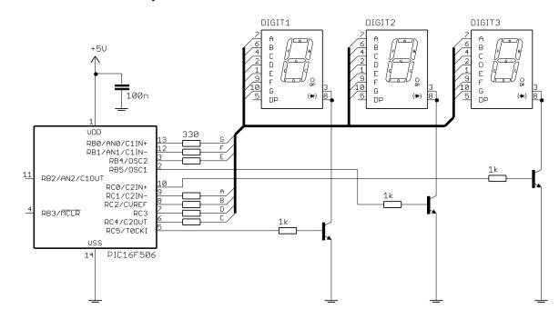
For that, transistors are usually used as switches, as illustrated below<sup>2</sup>:
