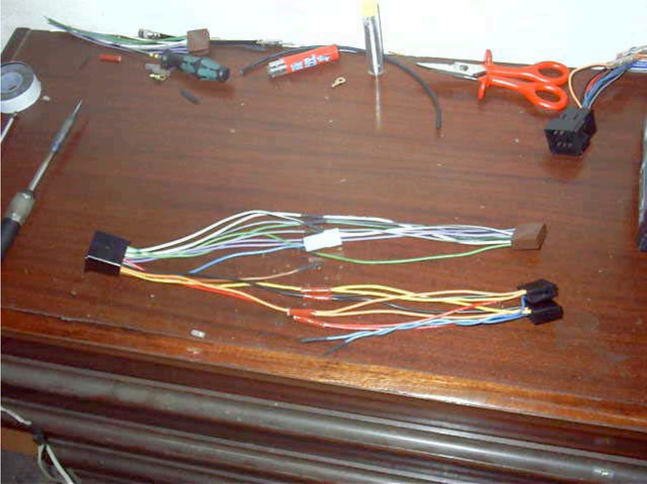
[On the left there is the female ISO plug that will be plugged to the car, on the right there are the three plugs for the new head unit]
