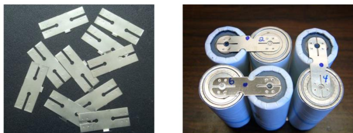
Fig. 20. Design alternatives for connecting tab with slot [6, 7].
