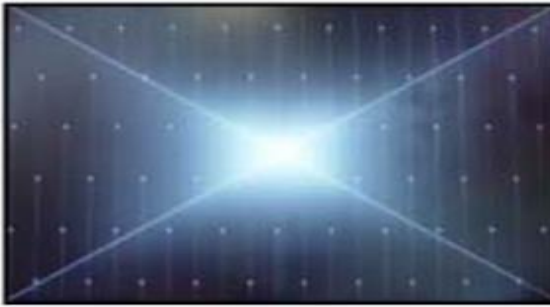
Solder defect, Short/Crack
