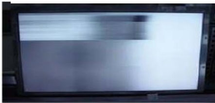
Horizontal Block Gate TAB IC Defect
