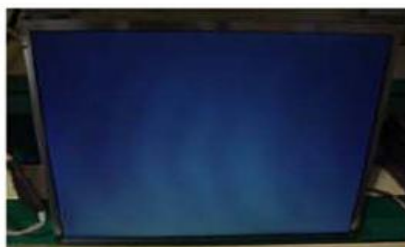
Panel Mura, Light leakage
