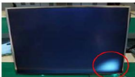
Panel Mura, Light leakage
