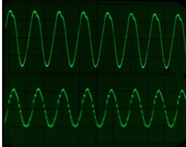
J1-1 Tx (top) 5v/Div & 20uS U101 Pin 7 Rx (bottom) .01V/Div & 20uS
