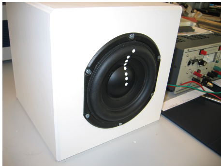
Figure 3-1: Woofer under test circumstances, with reflective tape to enhance laser reflectivity
