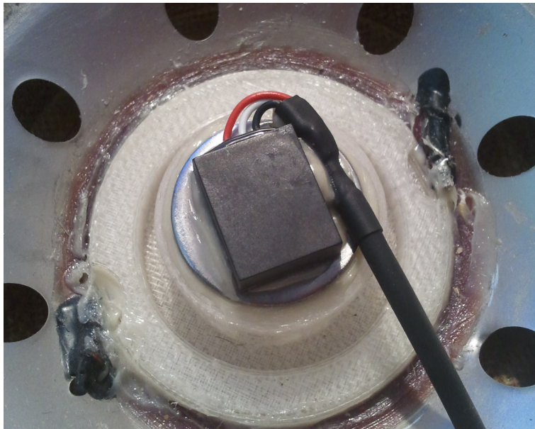
Figure 8-4: Physical implementation of new sensor mount
