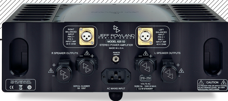
ABOVE: Balanced (transformer-coupled) inputs only, via XLRs, are joined by a pair of substantial screw-down cable connectors per channel. These are best suited to bare wire rather than 4mm or spade terminated loudspeaker cables
