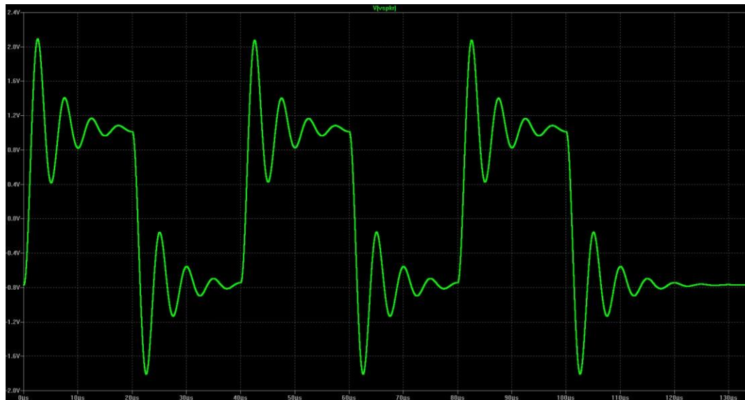
Plot 4 - nx-Amp output across 8 \Omega // 1 \mu F load with 25 kHz square wave input. The ringing is a consequence of the resonant circuit formed by the out inductor, cable inductance, cable capacitance and any speaker input capacitance. All amplifier outputs exhibit this ringing behavior on fast transients.
