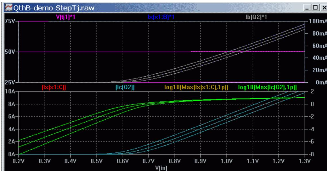
**Figure 1.2.1. Tj stepping demo jig for 0%, 50%, 100% interpolation**
