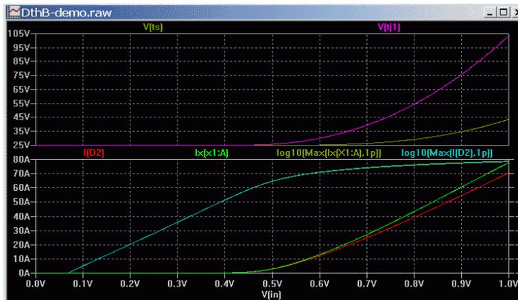
**Figure 3.3. Demo jig plots for the original MOSFET Id(M2) to the electrothermal subcircuit Ix(x1:D)**
