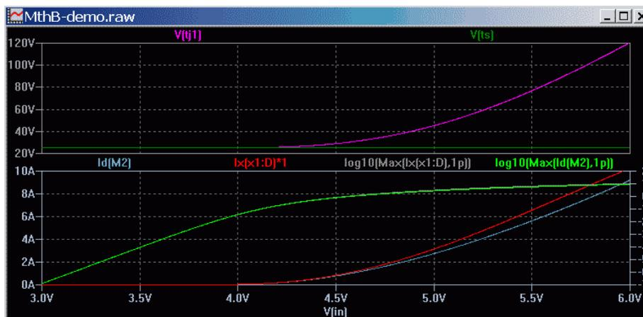
**Figure 2.3. Demo jig plots for the original MOSFET  $I_d(M2)$  to the electrothermal subcircuit  $I_x(x1:D)$**
