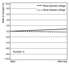
Characteristics were measured after applying a shock of 490 m/s $^{2}$  to the test piece 3 times each in 6 directions along 3 axes.
