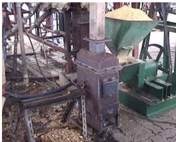
Figure 1.4: The improved briquetting system in operation
