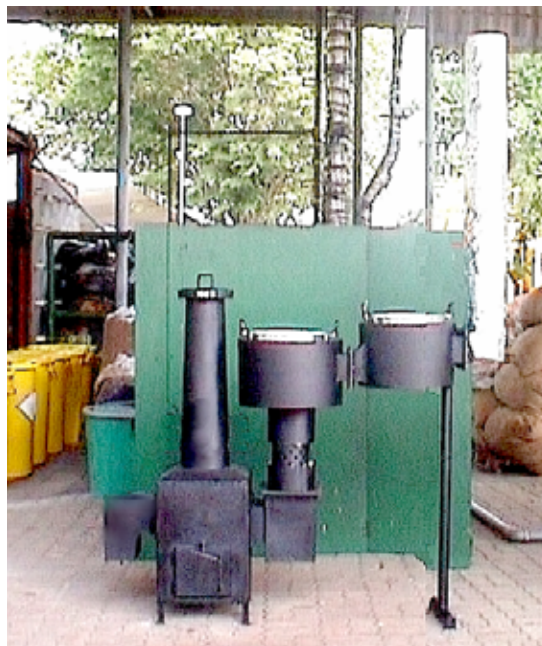
Figure 2.17: Fully assembled gasifier stove IGS2, with pot support
