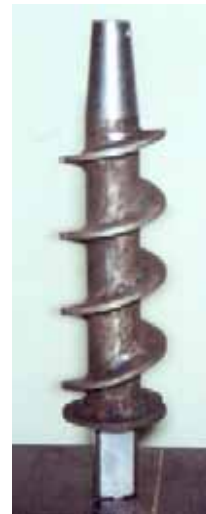
(iv). Completed screw, ready for installation
