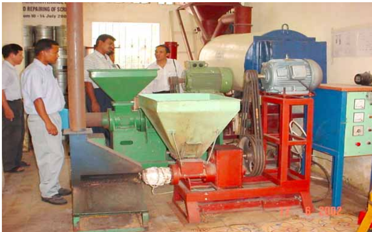
Improved briquetting machine, Vietnam
