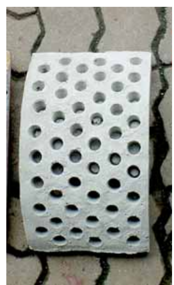
Figure 3.5: Pre-cast cylindrical sections for air inlet and gas outlet
