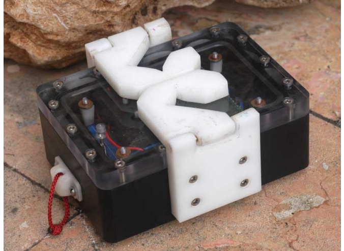
Figure 3: Compass suspended on line hangers (top). When not in use, hangers fold flat against compass body for stowing in pocket (bottom).
