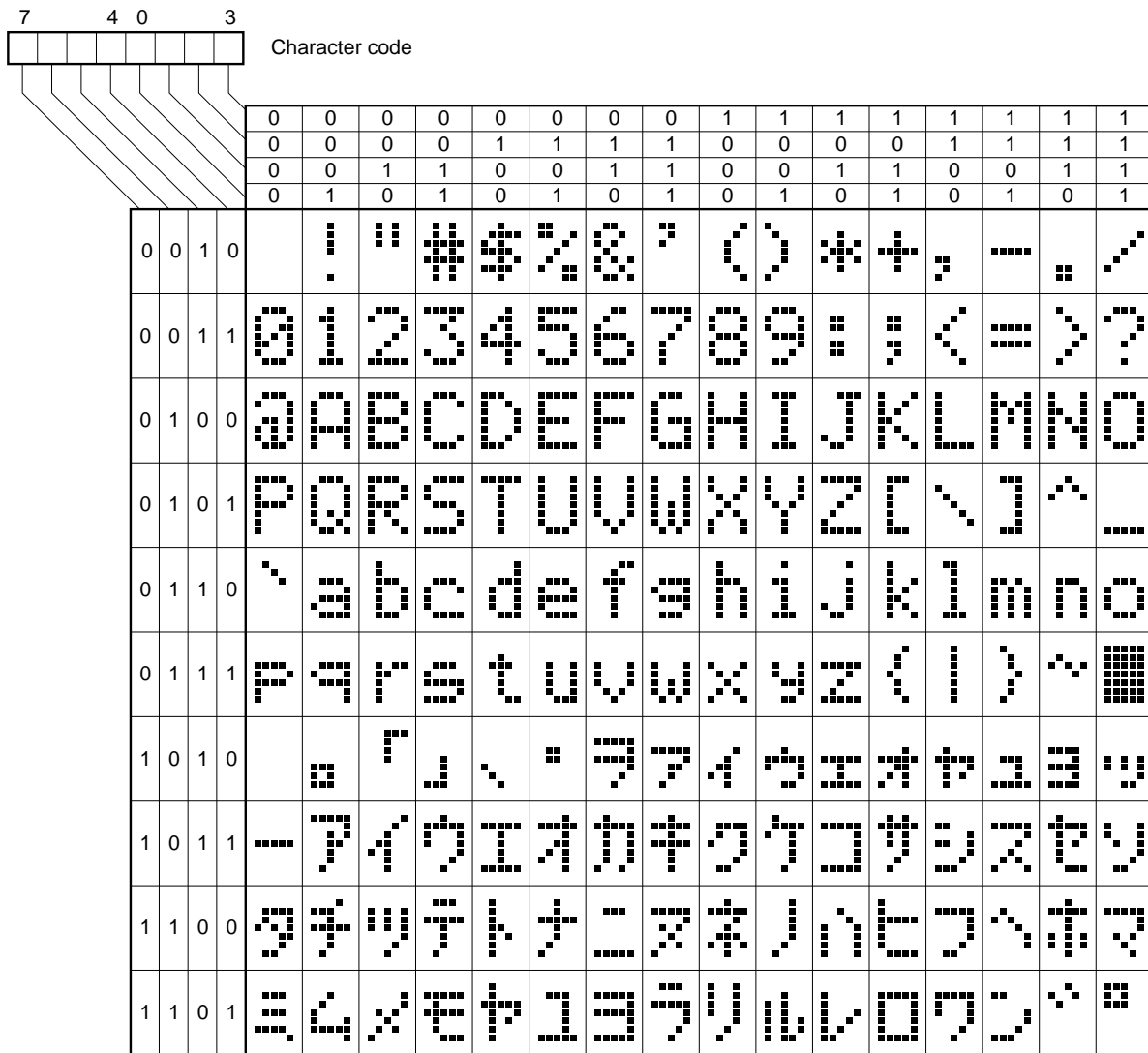
Figure 2-2. Character codes and Display Pattern (Standard ROM code: 001)
