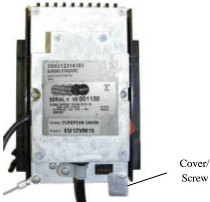
**Figure 21. Location of DIP-Switch Cover/Screw**
