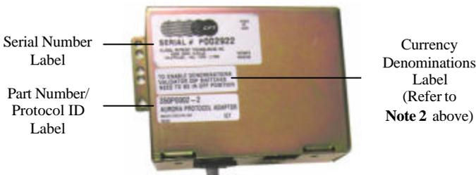
**Figure 10. Protocol Adapter Assembly – Label Identification**
