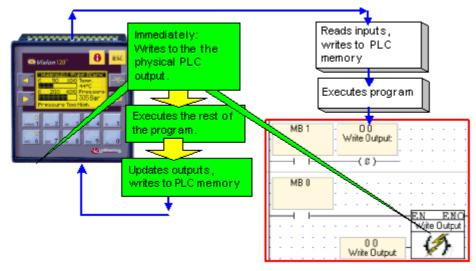
To use Write to Output, place it in a net after an activating condition and select the desired output.
