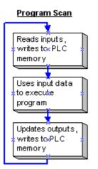
When the program encounters Write to Output, the program immediately writes the physical PLC output, then executes the rest of the program.
