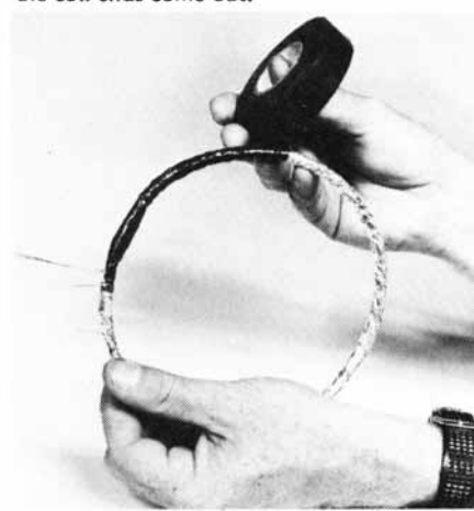
4: Cover the whole coil assembly with two more layers of insulation tape.
