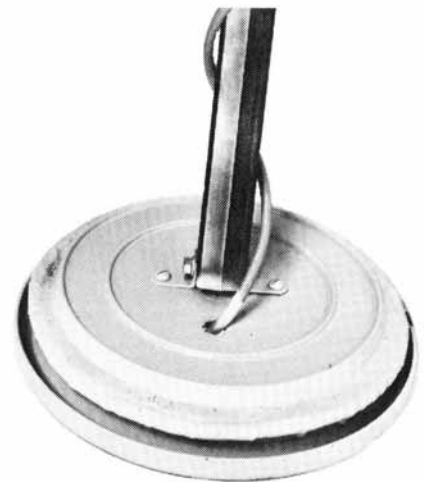
5: Press the assembled coil into the rim of the pot stand, terminate the wires as described and epoxy the coil to the pot stand.
