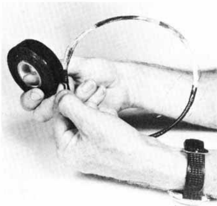
1: Having wound the coil as described, wrap it with two layers of insulation tape.
