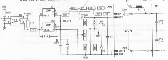
Overvoltage and undervoltage protection
