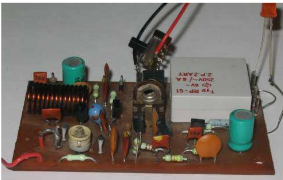
Receiver for transmitter in Circuit B
