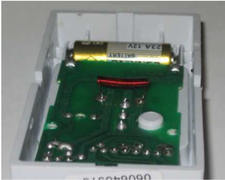
40 turn coil replacing the 1.5uH inductor
