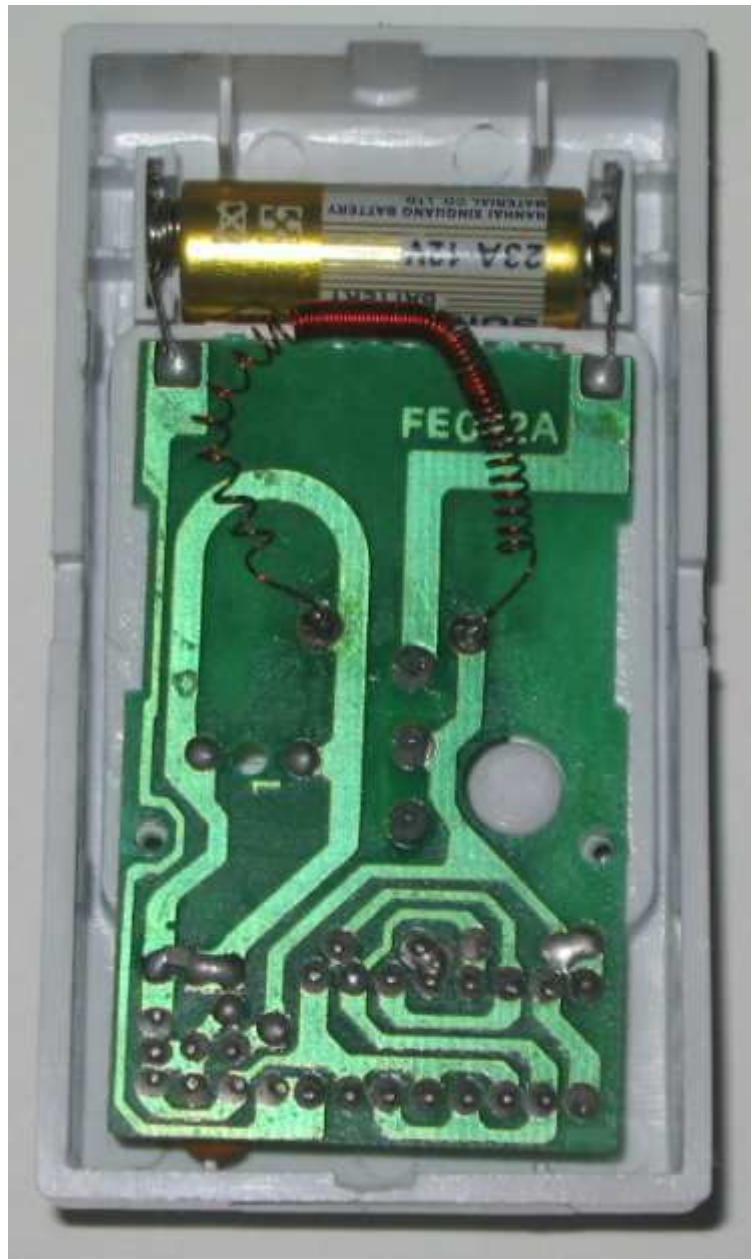
60 turn coil spread out to increase the range of the transmitter
