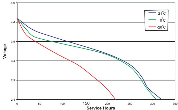
Typical Discharge at 20 ohm at various Temperatures
