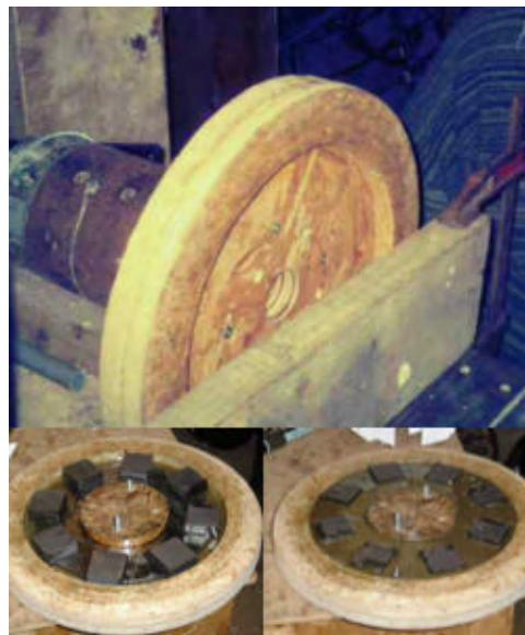
Rotor mould being made and used
