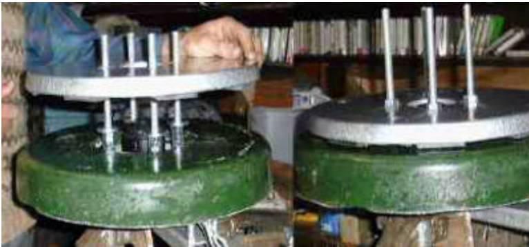
Fitting the front magnet rotor
