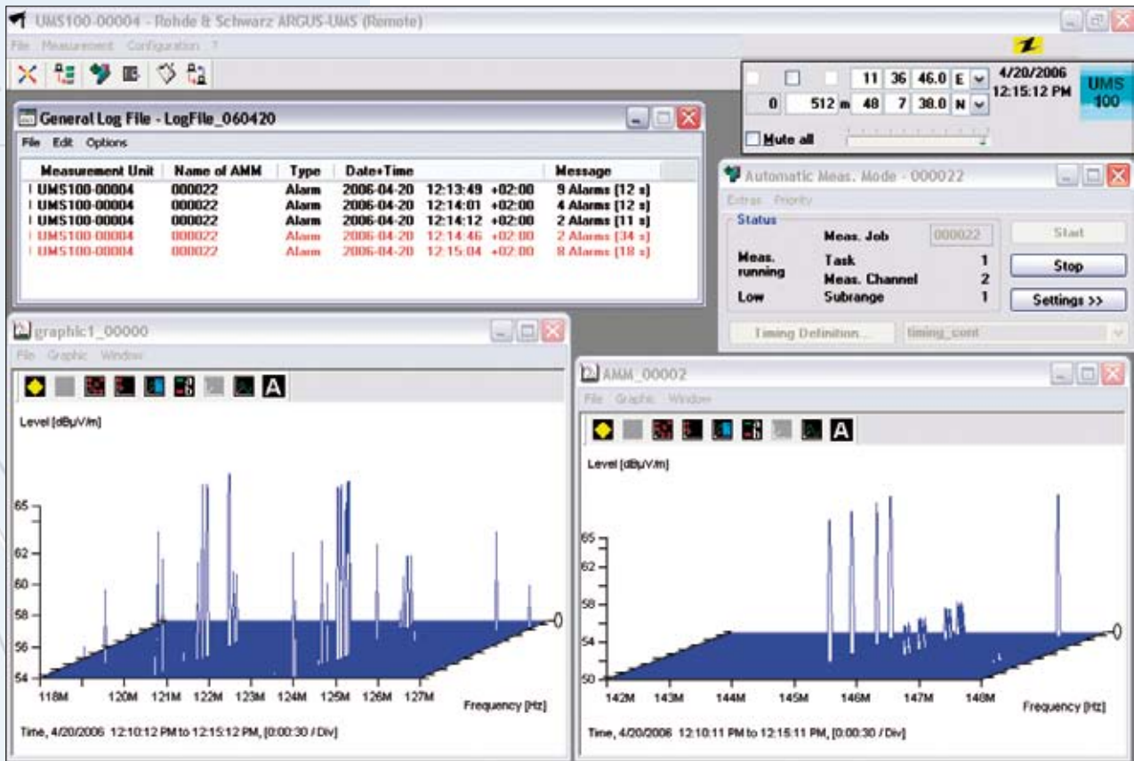
R&S® ARGUS-UMS control software window showing automatic measurement results and alarm log
