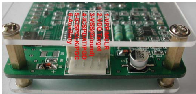
Figure 5 Right Side View (Debug/Program Port)
